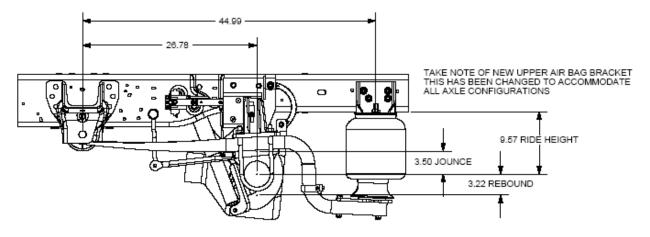
Note: The ride height is for the completed vehicle with body and components. See table below for correct vehicle dimensions. See following pages for the above views.
